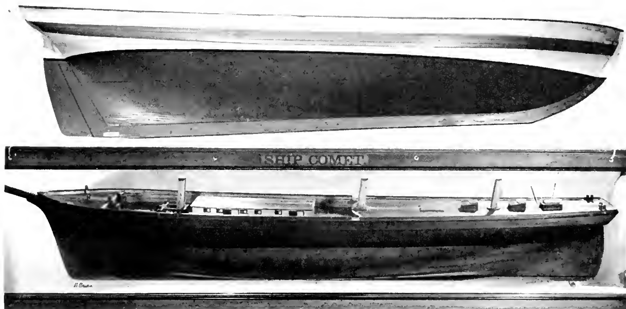
SEMIDECORATIVE LIFT MODEL (TOP) AND MIRROR-MOUNTED HALF-MODEL (BOTTOM). Models exhibited in shipyard offices commonly received the simple decorative treatment illustrated by the top model (USNM 315852; see p. 88). The stem, keel, post and rudder were usually secured to the back board, and masts and bowsprit stubs were sometimes attached. Occasionally a model was mounted on a mirror to give the illusion of a complete deck arrangement, as illustrated (bottom) by the half-model (USNM 76072; see p. 57) of the clipper ship Comet . (Smithsonian photos—top, 47607 d; bottom, 47608.)
